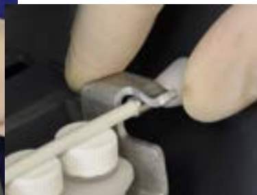
Tube blocking rod locked position
