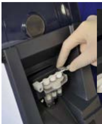
Tube blocking rod locked position
