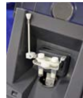
Correct and only position for 2 tubes
