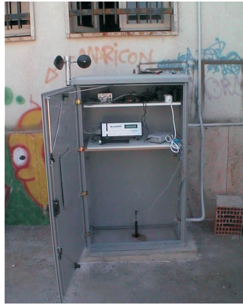
Figure 2: Monitoring station for radon in soil gas suited with GSM data Transmission in Modica
