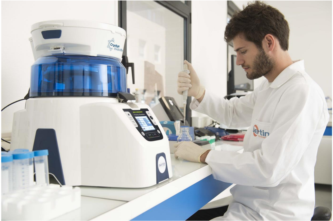
Photo Caption: Picture showing the Precellys® & Cryolys Evolution tissue homogenizer equipment on the bench
