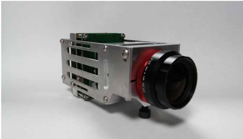
Figure 9 : CamSight, integrated camera modules for complex optronic systems. Copyright : Thomas Léaud
