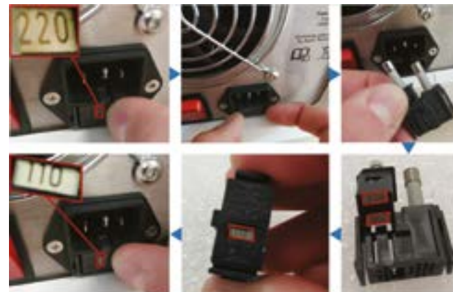
Figure 2: Instructions for adapting the device to the electric current (220V/110V)
