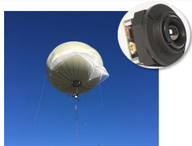
White Hawk tethered aerostat
