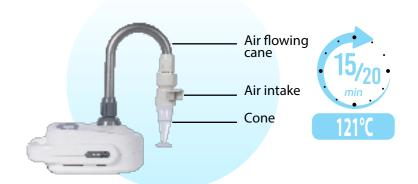
Autoclave the air flowing cane and air intake at 121°C, 15 psig (1 bar) for 15-20 minutes.
