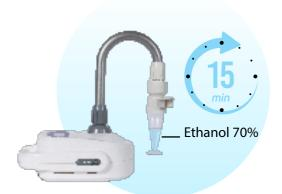
Run the Coriolis by filling the cone with ethanol at a flow rate of 300 L/min for 15 minutes.
