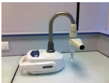
Coriolis \mu equipped with the air intake with 25mm connection
