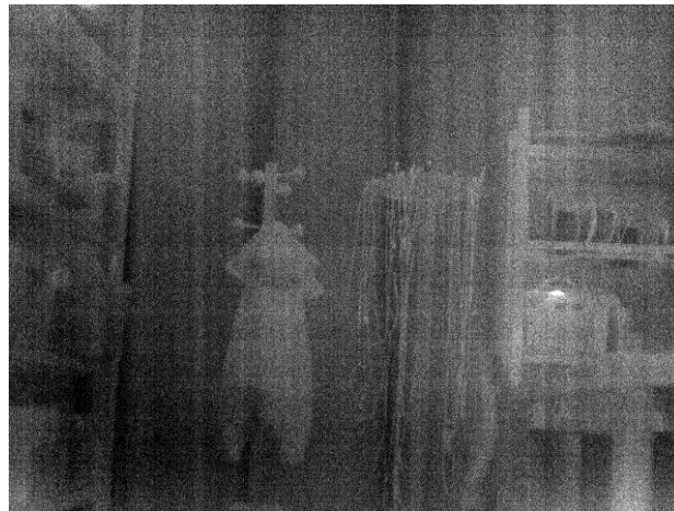
Figure 20 : Original image with low contrast and high noise (no AHC)
