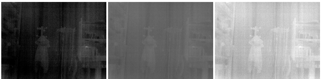
Figure 20 : Original image with low contrast and high noise (no AHC)
