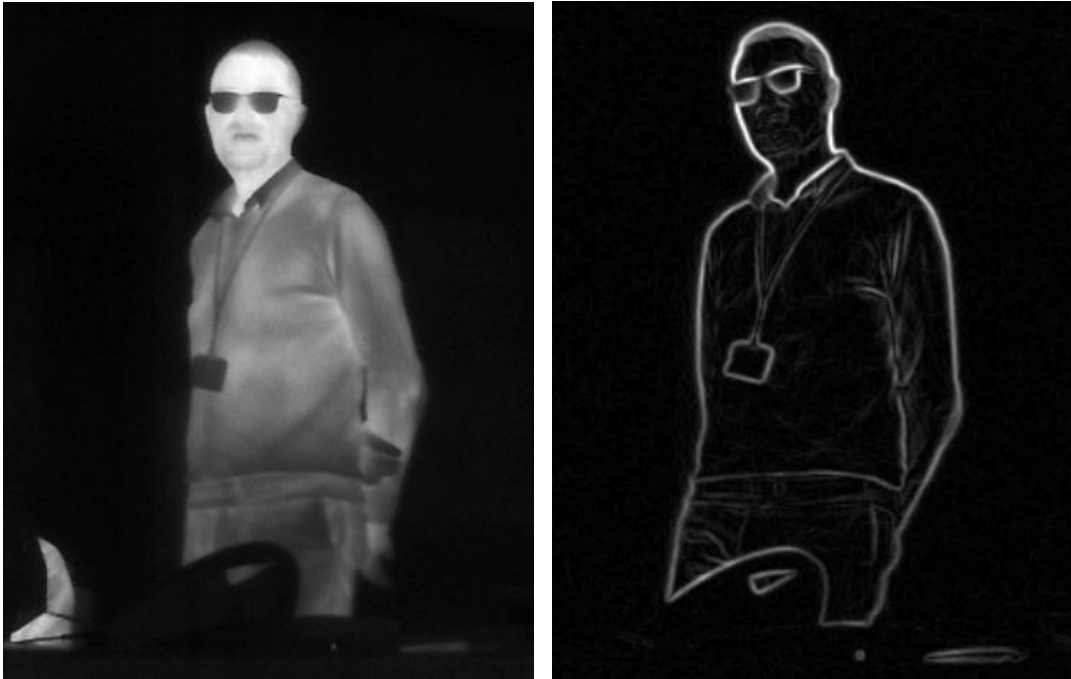
Figure 18: Contouring filter turned off (left) / on (right)
