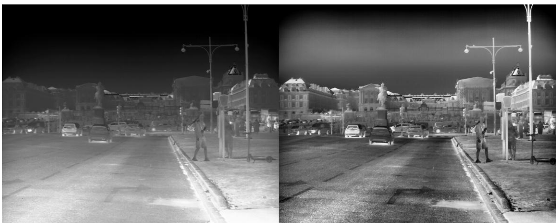
Figure 19: CLHE algorithm (left) / CLAHE algorithm (right)
