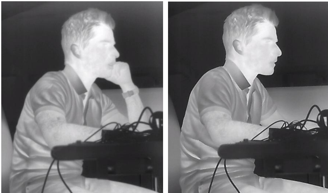
Figure 17: Sharpening filter turned off (left) / on (right)
