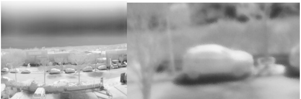
Figure 31: CamSight HD with 8.5mm lens: Left picture – Zoom x1 / Right picture – Zoom x8
