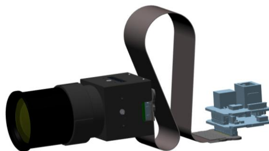
Figure 19: 3D rendering of the CamSight HD with a 15 mm lens and the GigE Vision interface
