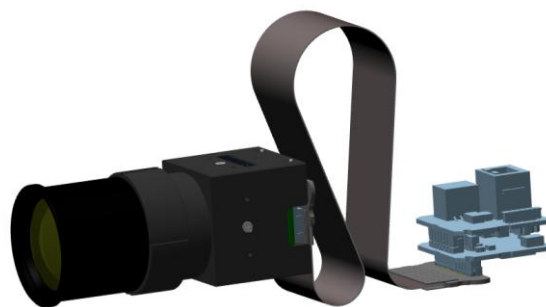
Figure 16: 3D rendering of the CamSight HD with a 15 mm lens and the GigE Vision interface
