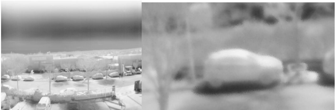
Figure 33: CamSight HD with 8.5mm lens: Left picture – Zoom x1 / Right picture – Zoom x8
