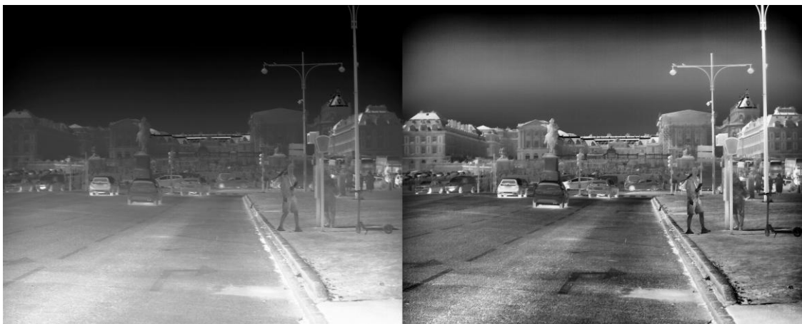
Figure 30: Left picture - CLHE / Right picture – CLAHE
