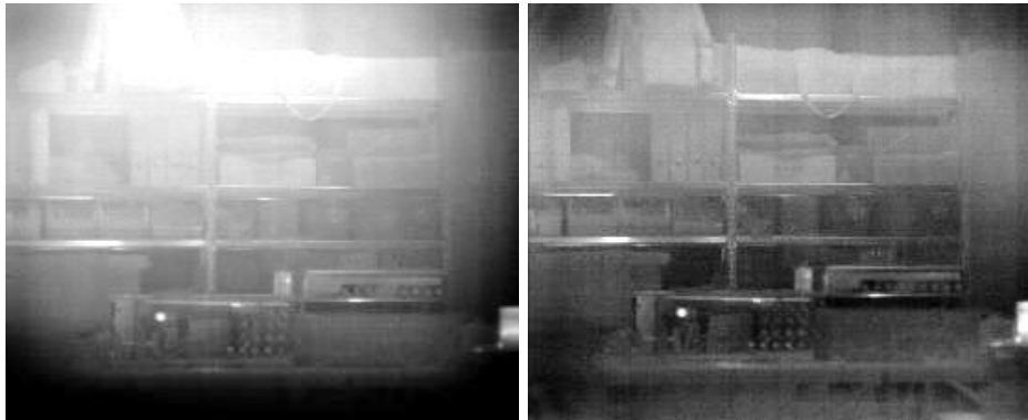
Figure 28: Left picture - vignetting correction OFF / Right picture - vignetting correction ON
