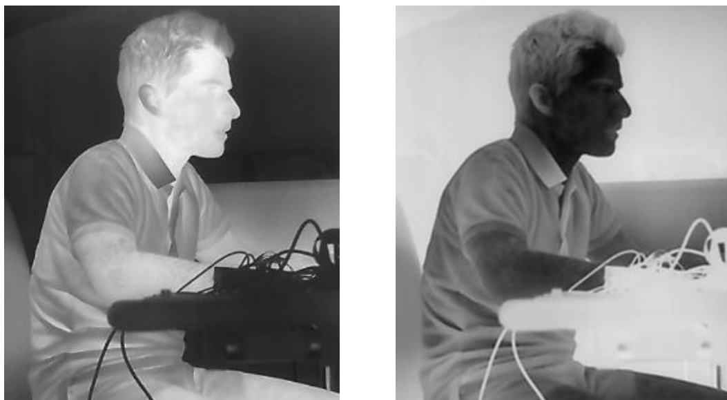
Figure 31: Left picture - White Hot / Right picture - Black Hot
