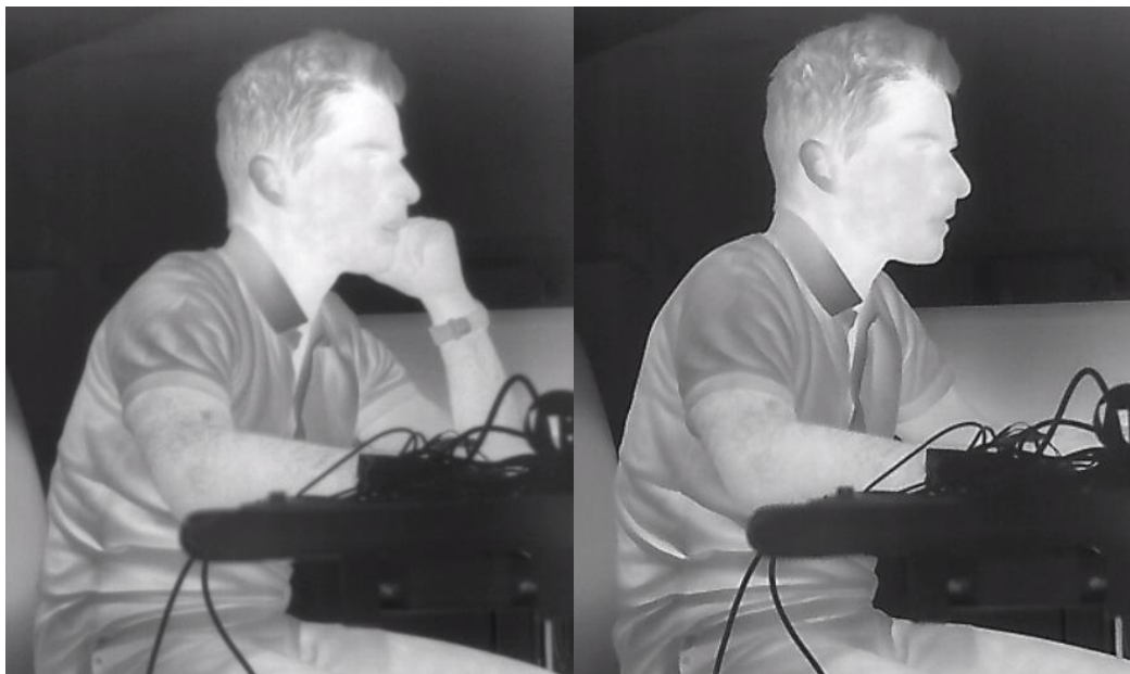
Figure 15: Left: sharpening off / Right: Sharpening on
